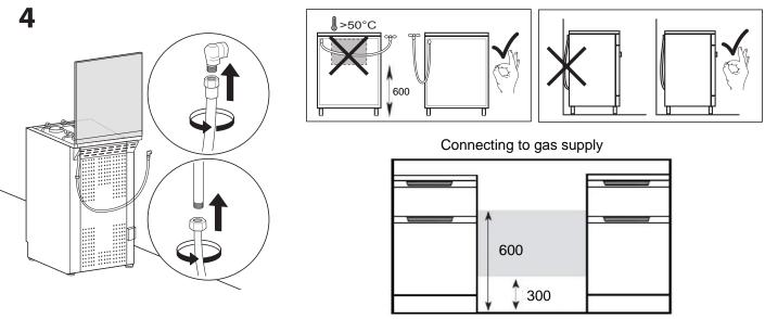
Gas hose connection point must be installed within the shaded area
