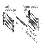
2. Choose which shelf to use with the sliding rack. Paying attention to the direction in which the sliding rack is to be extracted, position joint A and then joint B on the rail.
