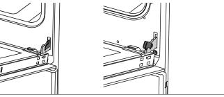
Later, close the opened oven door so that it will be in a position to contact with hinge lock.
