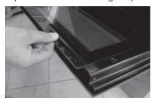
Open the door fully and unscrew the two screws securing the glass panel so that the securing brackets can be turned. There is no need to remove the screws completely.
