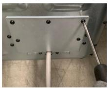
Assemble cover and tighten screws.
