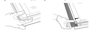
**2.** Lift and firmly hold the inner glass with both hands, remove it and place it on a soft surface before cleaning it.
