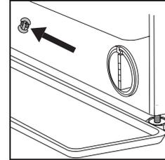
Remove the stopper of the "emergency drain hose" at the end of the hose and let the water flow into the container.
