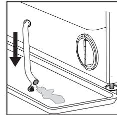
3. Turn the exhaust filter handle and pull it out of the housing. When the container of plinth is full with water, plug the stopper to the hose end, and reinsert the small hose in the washing machine's base. After, empty the container.
