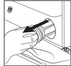
5. Clean the water filter: remove residues in the filter and clean it under running water.
