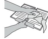
6. Reinsert the accessory by placing the back part on the projections shown in figure, then refasten the handle of the accessory to the clasps above.
