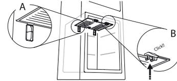
7. Reinsert the upper drawer and close the door of the freezer compartment.
