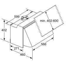
measurements in mm
