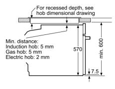
measurements in mm
