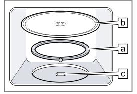
2. Engage the turntable b in the drive c in the centre of the cooking compartment floor.
