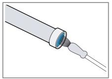
**3.** Connect the water inlet hose and check for leaks.
