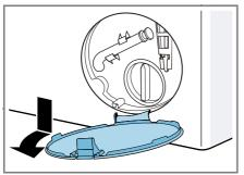
**6.** Slide a sufficiently large receptacle under the opening.
