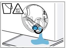
9. Firmly press on the sealing cap.
