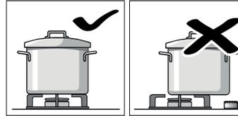
Always centre the pan over the burner, not to one side. Otherwise it could tip over. Do not place large pans on the burners near the control knobs. These may be damaged by the very high temperatures.
