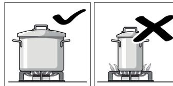
Use pans which are the right size for each burner. Do not use small pans on large burners. The flame must not touch the sides of the pan.
