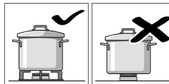
Place the pans on the pan supports, never directly on the burner. Make sure that the pan supports and burner caps are correctly positioned before using the appliance.
