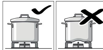
Do not use damaged pans, which do not sit evenly on the hob. Pans may tip over. Only use pans with a thick, flat base.
