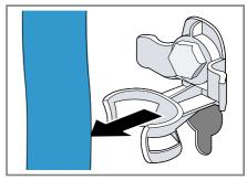
Unscrew ① and remove ② all screws for the 4 transit bolts with a WAF 13 wrench.
