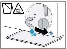
8. Firmly press on the sealing cap.
