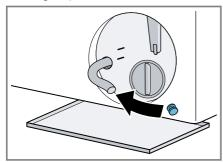
**8.** Insert the drain hose into the holder.
